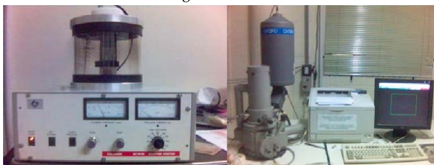
Figure 1. The photo of the sample coating equipment as the preliminary treatment (a), and the SEM-EDX equipment (b)
