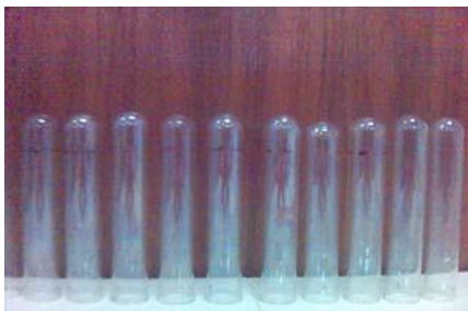
Figure 6. Ten glass tubes immobilized with thin layers of TiO 2
