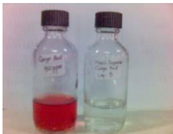
Figure 13. The degradation results of Congo Red were irradiated with UV light with TiO_2 for 240 minutes
